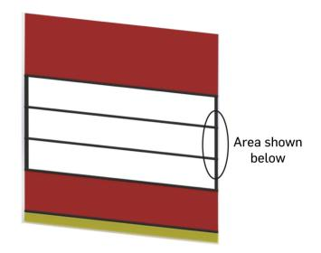
**STEP 3:** Remove the old section by removing existing 1/8" roll pins located at each end of upper and lower windbars. Use a nail punch or other punch tool to pound the roll pins out.
