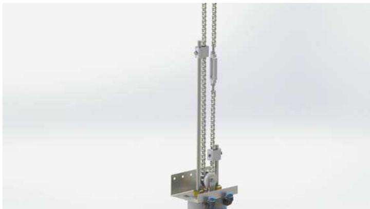
1. Start with door in the CLOSED position. This will raise the piston rod that is furthest from the wall and lower the piston rod closest to the wall.
